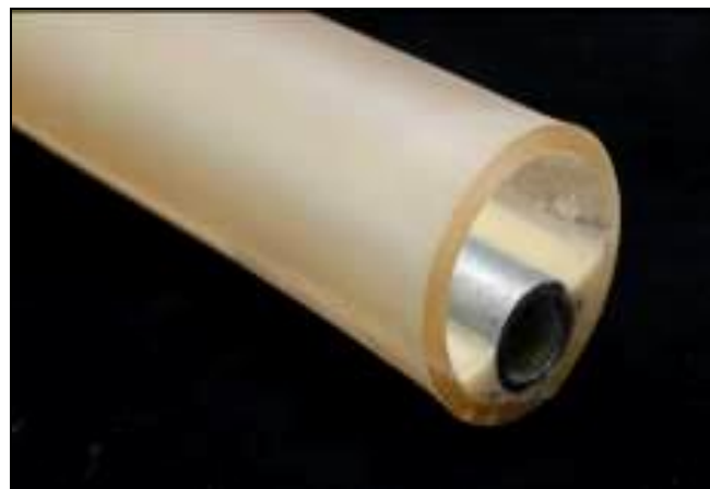
Fig. 5. A soft perch buffers pressure peaks on the keel bone. In this prototype this effect is achieved by an air cushion between the hard core and the flexible shroud.
