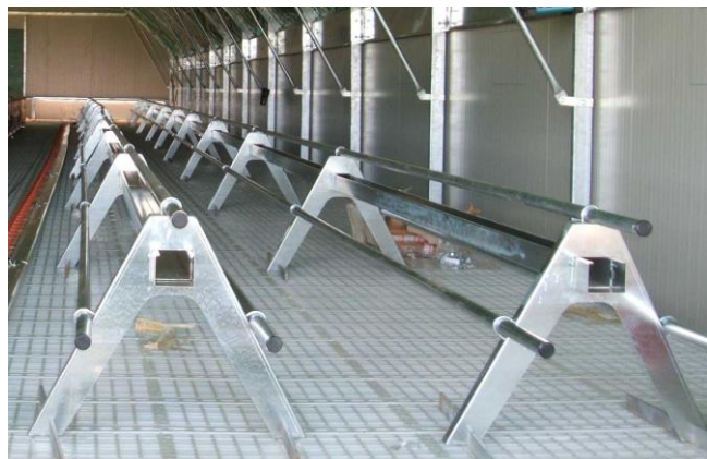
Fig. 4. A-frame style perch, incorporating feed track (courtesy of Newquip/Big Dutchman)
